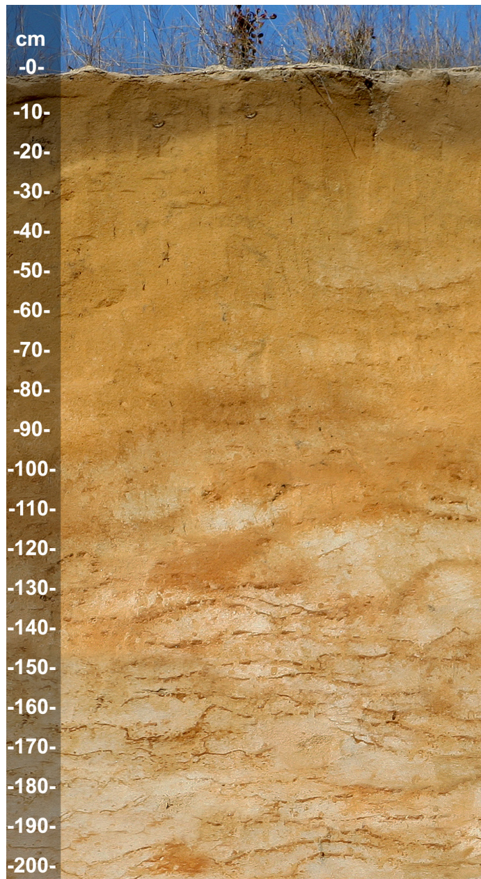
Figure 3-23: Profile of a soil that has an argillic horizon composed of lamellae. (Photo courtesy of John Kelley)
