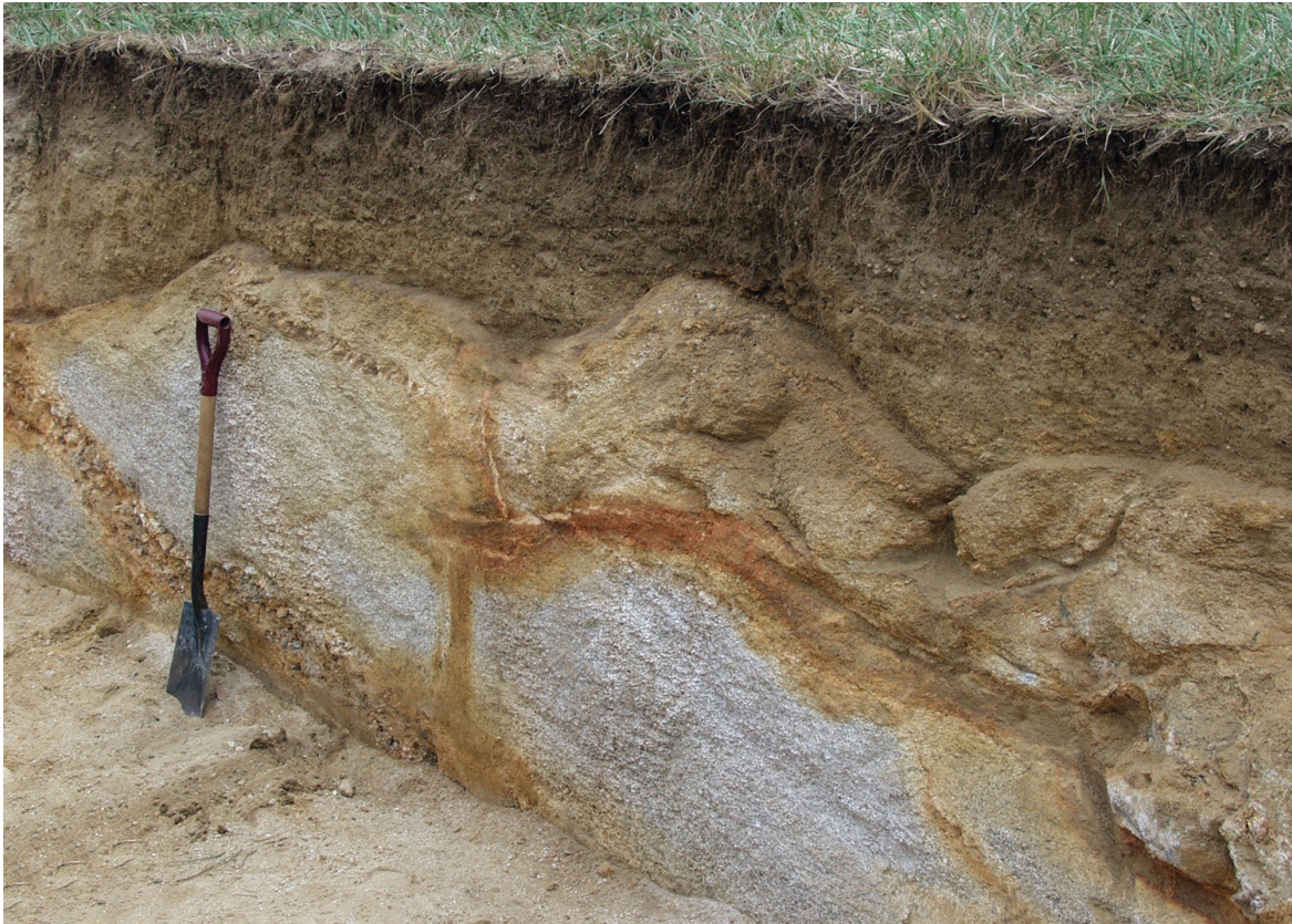
Figure 3-30: Soil profile with an abrupt wavy boundary at the paralithic contact. The paralithic material below the contact is relatively soft, weathered bedrock that can be dug with a spade. (Photo courtesy of John Kelley)
