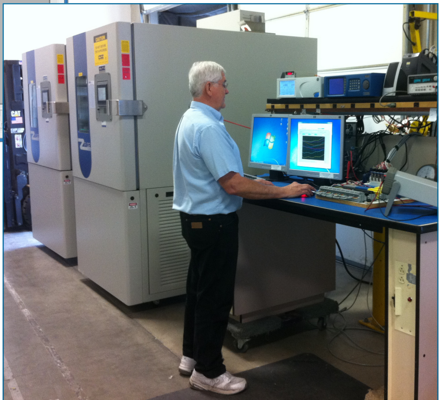
John Weeks uses Labview software to monitor the status of the pressure transducers under test. The two, new environmental chambers are at the left.
