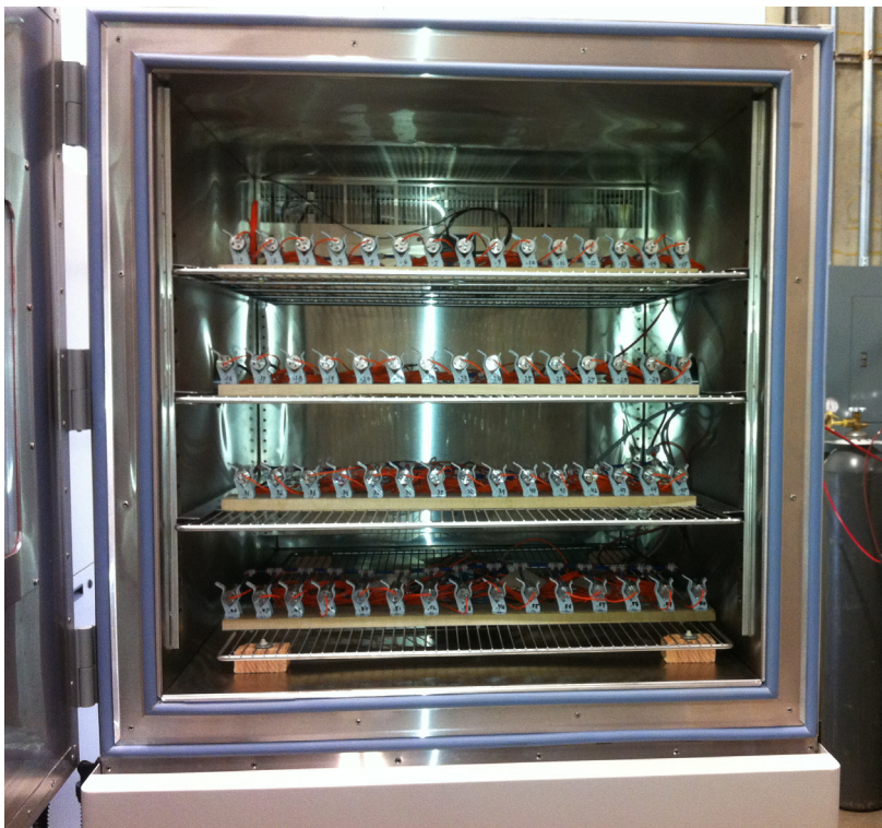
The interior of one of the new environmental chambers at EMF. Each chamber can process 60 pressure transducers.
