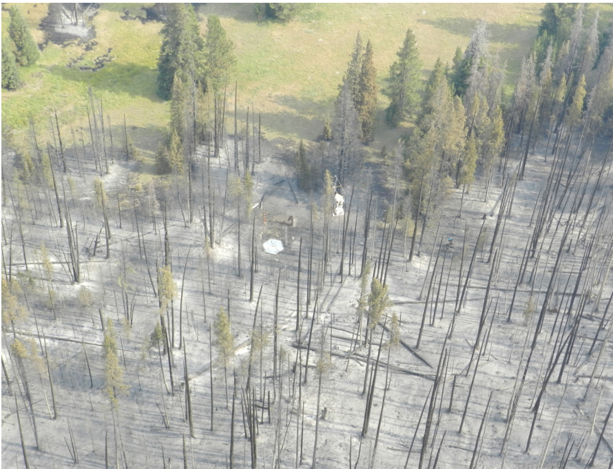
Younts Peak SNOTEL site in northwest Wyoming. The hexagonal footprint of the snow pillow is apparent in the center of the photo.
