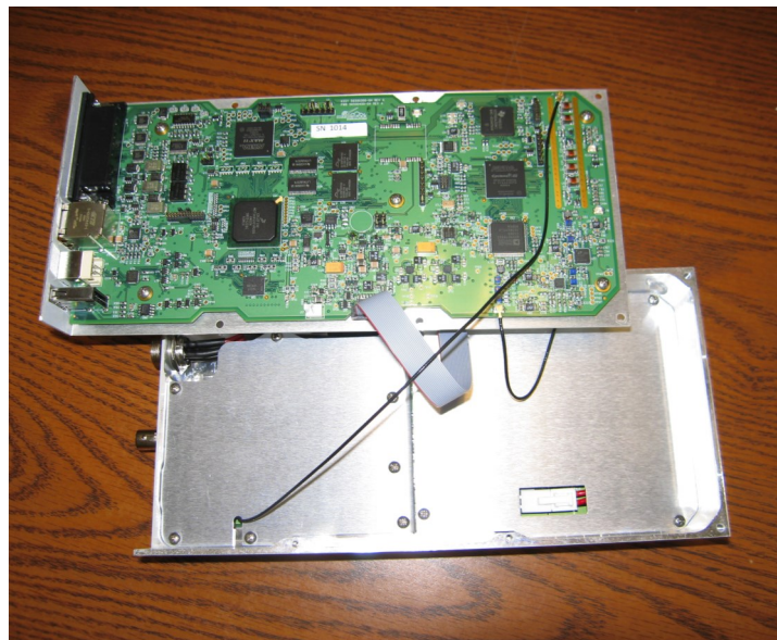
The MRC 565 features new circuit boards, software-defined functions, lower DC power consumption and a smaller footprint.
