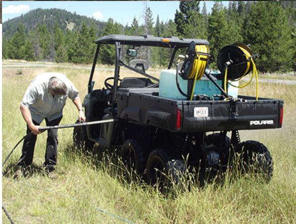
Thoroughly wash the vehicle, especially areas that hold mud with seed and debris. Longer wash times are more effective for removing weed seed. Photo MNWEC.
