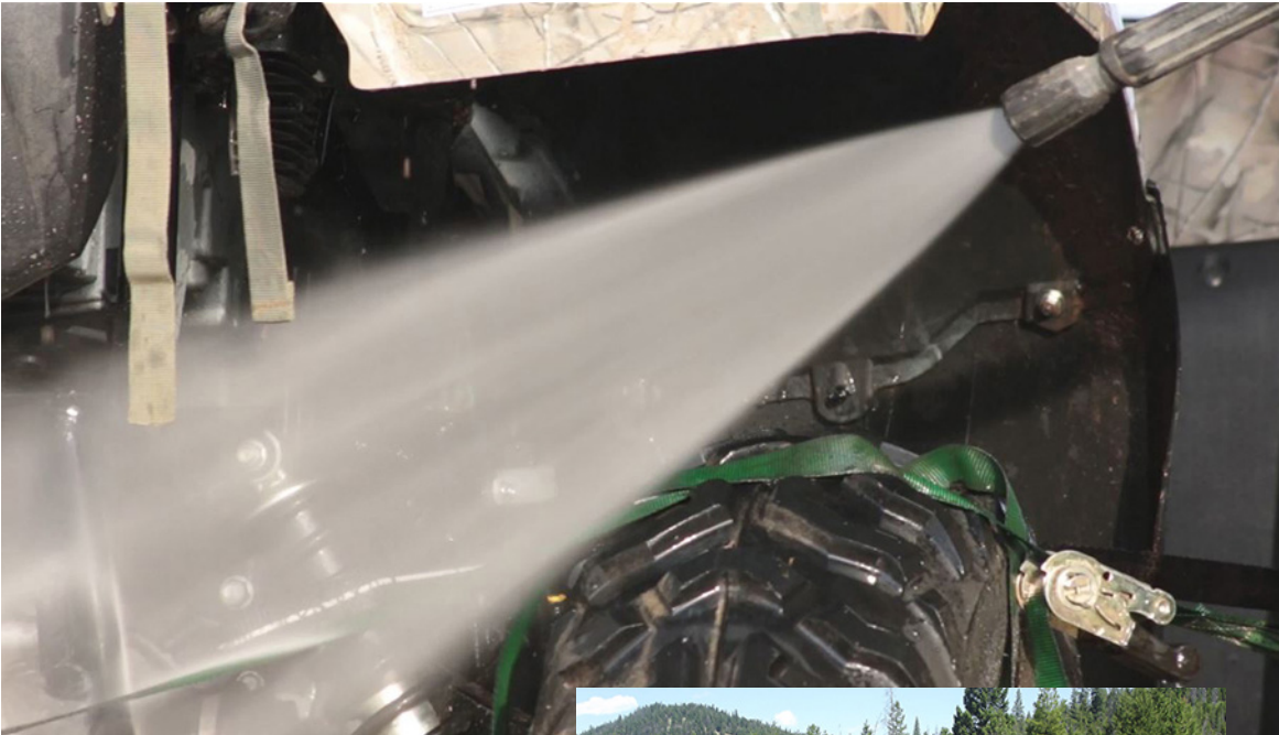
Thoroughly wash the vehicle, especially areas that hold mud with seed and debris. Longer wash times are more effective for removing weed seed. Photo MNWEC.
