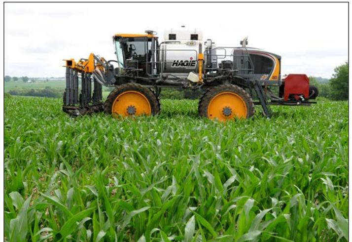
*A high-clearance sprayer is used by a northeast Iowa farmer to apply cover crop seed between corn rows.*
