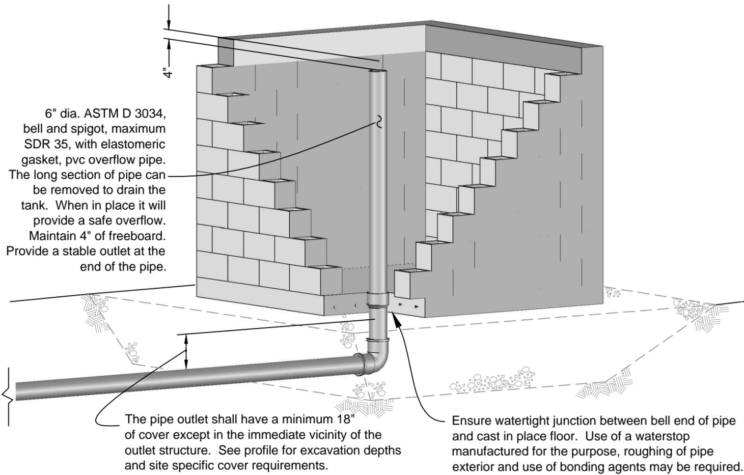
**Cutaway Showing Removable Internal Overflow Pipe**
