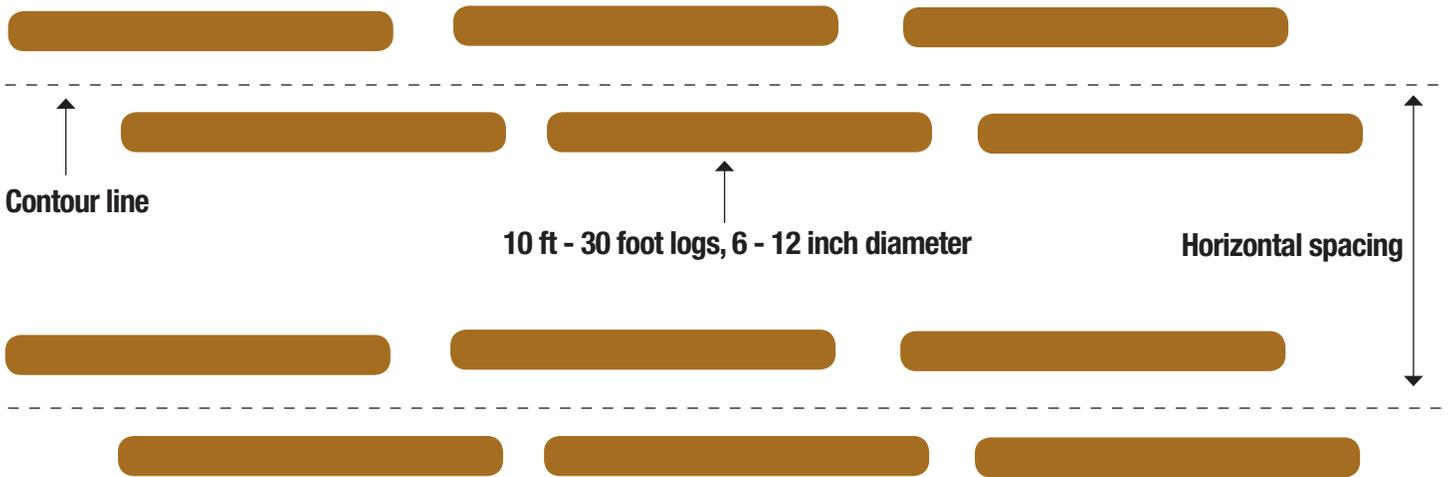
**Fig. 2 - Typical log & bedding detail**
