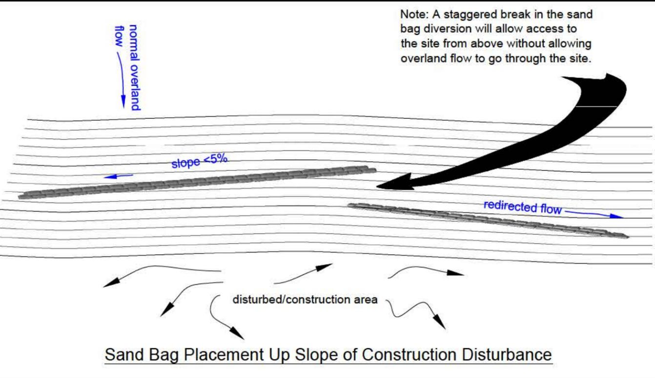
**Sand Bag Placement Up Slope of Construction Disturbance**
