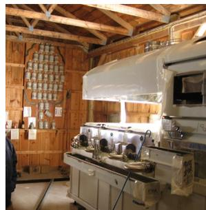
**Maple Syrup Reverse Osmosis, Steam-enhanced Pans, and Evaporators:** Farmstead energy improvements to reduce evaporation time includes new or replaced reverse osmosis system, new membrane, steam-enhanced pans, and replacement of inefficient evaporators for energy savings of up to 75 percent.
