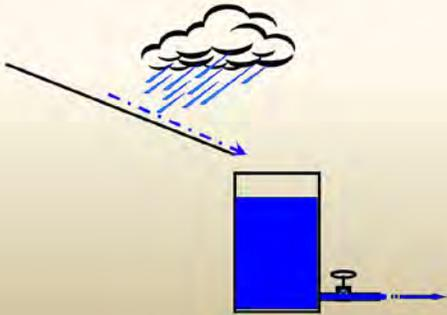
A **water harvesting catchment** is a facility to collect and store runoff from precipitation. Rainwater is very clean. Diverting the first few millimeters of rainfall (the “first flush”) from the catchment will avoid most of the contaminants.
