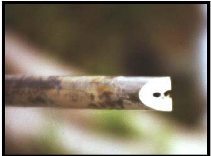
Pictures of the stainless steel nozzles that were welded to 1/2 in steel pipe. The stainless steel is expected to increase the life of the waterjet. A machinist built the pipe, handle, and nozzles as a single unit. The ball valve is added by the end user.
