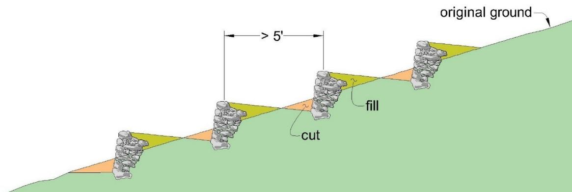
Figure 2: Horizontal Separation Between Adjacent Rock Wall Terraces
