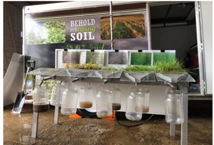
*The NRCS rainfall simulator is shown after two inches of rain. The front buckets represent runoff, while the back buckets represent infiltration. The plots from left to right are conventional tillage with no cover crop, till with cover crop, no-till with cover crop, continuously grazed pasture and rotationally grazed pasture.*
