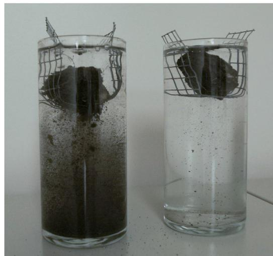
Figure 1.—Rainfall simulator and slake test demonstrations (pictured) show the consequences of soil management decisions.
