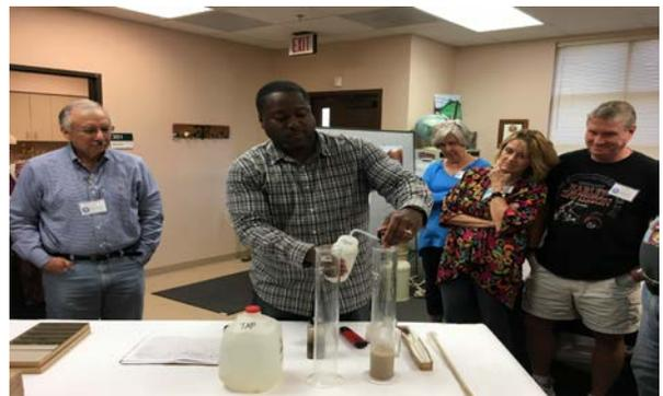
Cody Langston, Soil Scientist, Rosenberg, Texas, demonstrates the use of a hydrometer and sedimentation jar for determining soil texture.
