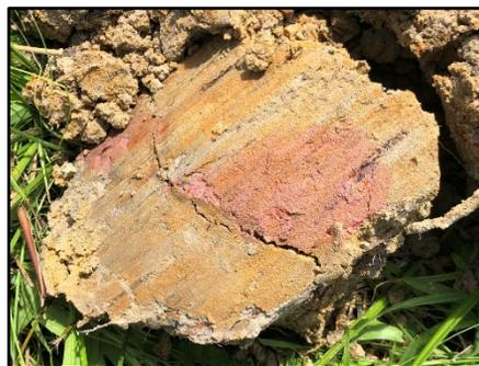
Reduced iron ( $\text{Fe}^{2+}$ ) shown by strong reaction (red areas) to alpha-alpha-Dipyridyl solution applied to a soil ped.
