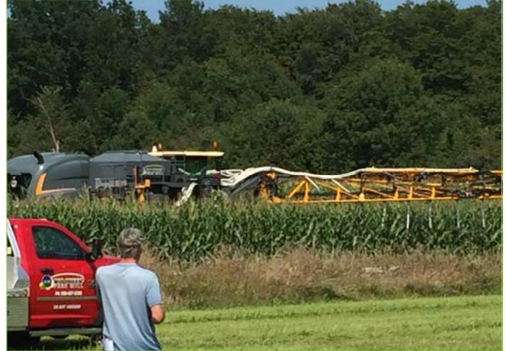
Rio Creek Feed Mill provided a Hagie high clearance sprayer, equipped with a cover crop seeder, for field day participants to view. Producers were able to watch the seeder in action and Rio Creek Feed Mill staff were on hand to answer questions about the seeder.
