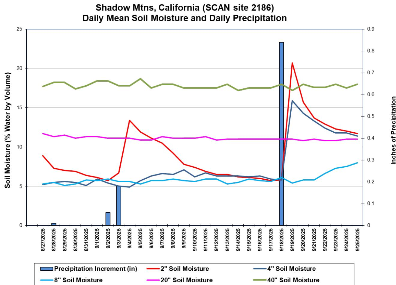
This chart shows the precipitation and soil moisture for the last 30 days at the [Shadow Mtns](#) SCAN site in California. A pronounced increase in soil moisture was recorded at the -2 and -4-inch soil sensor depths after the site received 0.84 inches of precipitation on September 18. Total precipitation for the 30-day period was 1.09 inches.
