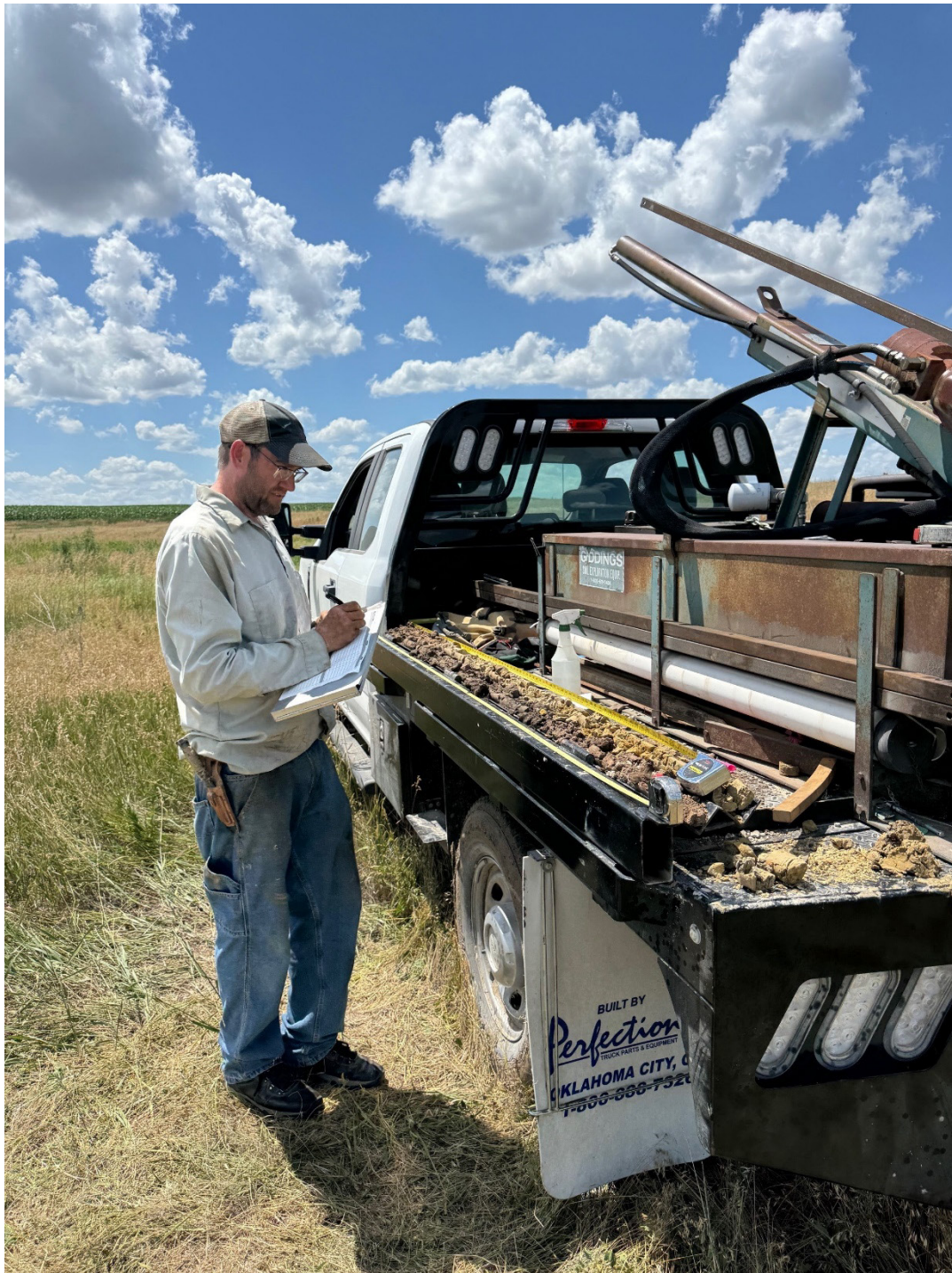
Figure 1.—Still and Scott used a pickup mounted hydraulic soil probe to collect a soil core sample approximately 17-feet long and then determined and recorded the properties of the soil.
