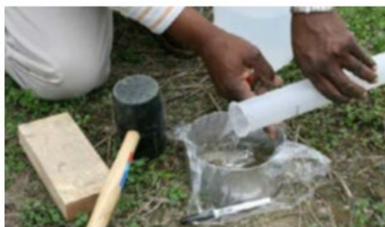
Figure 5: Preparing soil infiltration test
