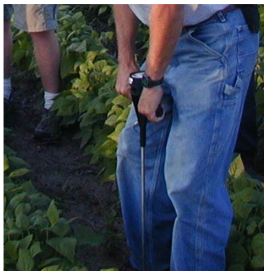
Figure 6: Applying slow, steady pressure when pushing penetrometer into soil.
