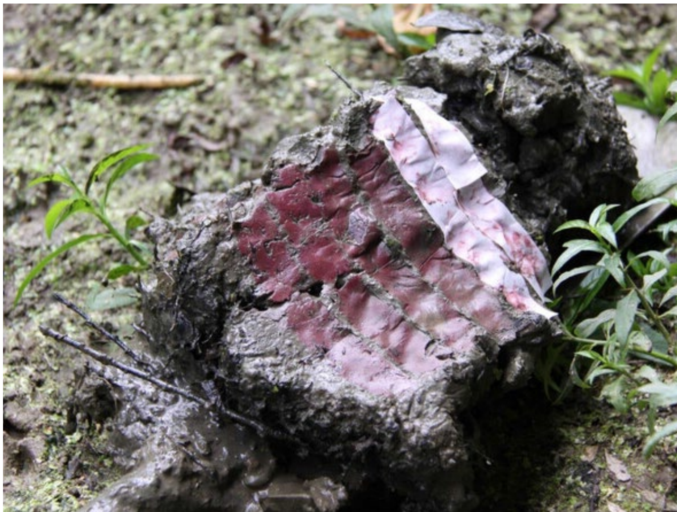
Figure 9.—A soil exhibiting anaerobic conditions through the application of alpha-alpha dipyridyl dye embedded in paper test strips. Note that the positive reaction results in a red or pink color occurring over approximately 80 percent of the soil surface, which is above the 60 percent required to document anaerobic conditions in HSTS studies (Berkowitz et al., 2021).
