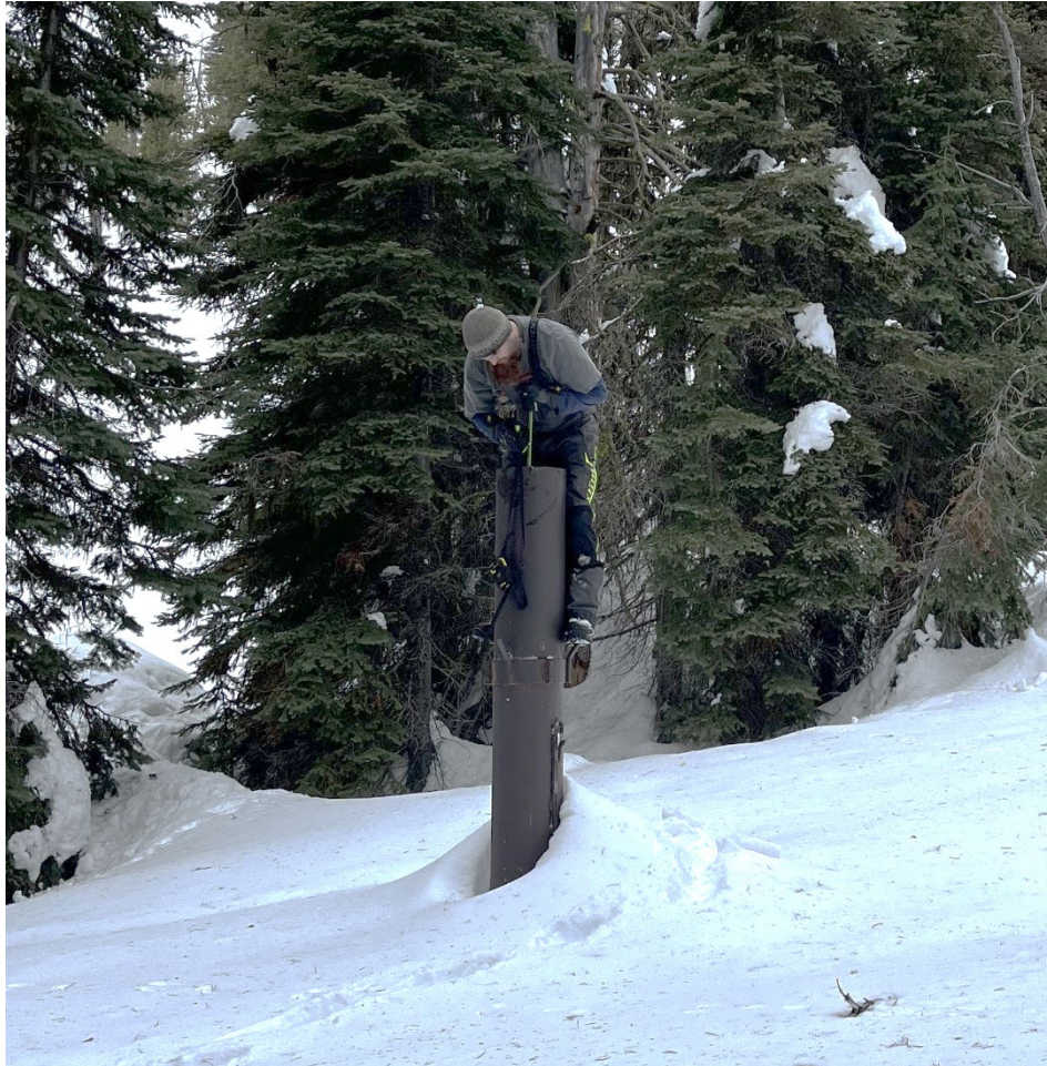
Snow surveyor Justin Byington works to clear a snow plug out of the precipitation can at Deadwood Summit SNOTEL site. Photo courtesy of Earl Adsley
