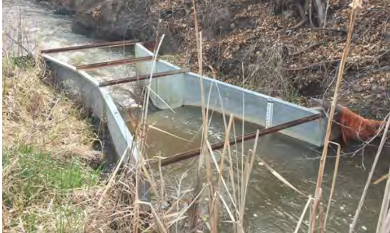
Figure 46. Three-foot Parshall flume just downstream of the flow control gate
