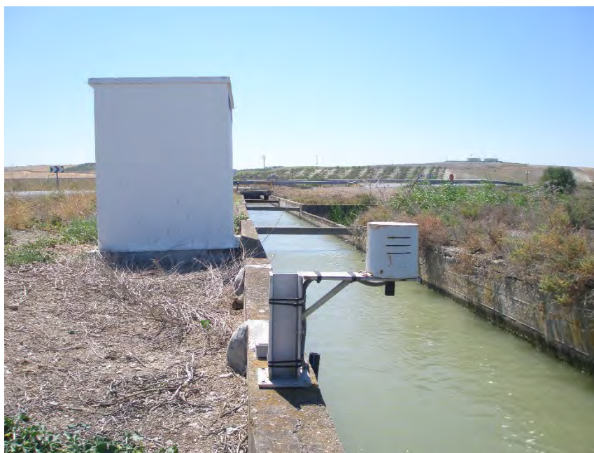
Figure 82. Another example of a simple ultrasonic water level measurement – this bracket does not appear to have enough overhang to eliminate obstructions of the cone-shaped sound path. Note the white, vented enclosure for temperature control.
