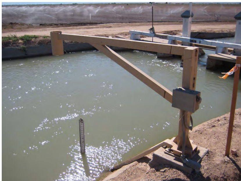
Figure 81. Example ultrasonic water level measurement with retractable (swinging) bracket and staff gauge at Imperial Irrigation District. The RTU is not shown.
