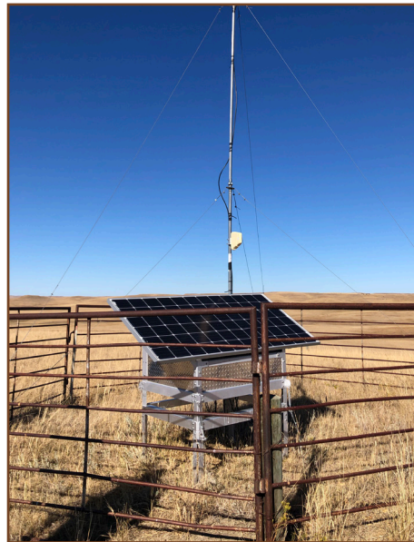
Example of a base station being protected by cattle panels. (Photo by Emily Rohrer).
