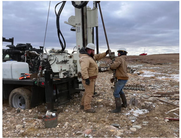
Above: Hayes Durbin, Iowa NRCS Engineer Technician inserts the center bit rod into a hollow-stem auger in preparation to drill test hole during t I am joined by South Dakota NRCS staff. The center bit rod and hollow-stem auger are used to drill a borehole to a desired depth. Once at that depth, the center bit rod is removed and the SPT is performed within the hollow-stem auger.
