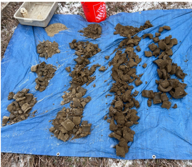
Above: Roughly 20 ft of soil samples taken directly off the flights of 4" outside diameter solid-flight augers from test hole #1. These samples will be analyzed at the National Design, Construction, and Soil Mechanics lab in Lincoln, NE for their engineering properties and qualities.
