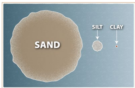
Relative sizes of sand, silt and clay
