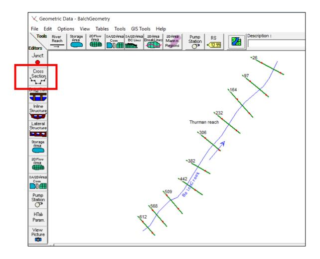
Inspect the cross sections to verify geometry imported correctly. Compare to section views in CAD. Sometimes, if you don't Flip the \*.geo file, the cross sections will be reversed or the alignment reversed. Carefully look through several sections to verify. Look at more cross section by using the black arrows by River Sta.
