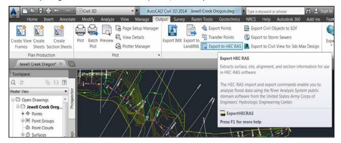
Select the surface you want to sample from, and the alignment and samples lines just created. Site = None. Enter the River Name. Check River Banks box — when you click Left, CAD will prompt you to select a polyline or alignment — select your Left overbank alignment or polyline. Do the same for Right bank. Then Click Export. Make note of where you save the file.
