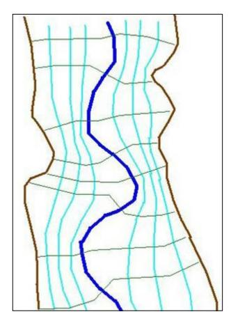
It takes a little bit of practice to do this correctly, and most of the time some trial and error, but as long as you remain perpendicular to the flow lines and don't intersect, you'll have a good set of cross sections.
