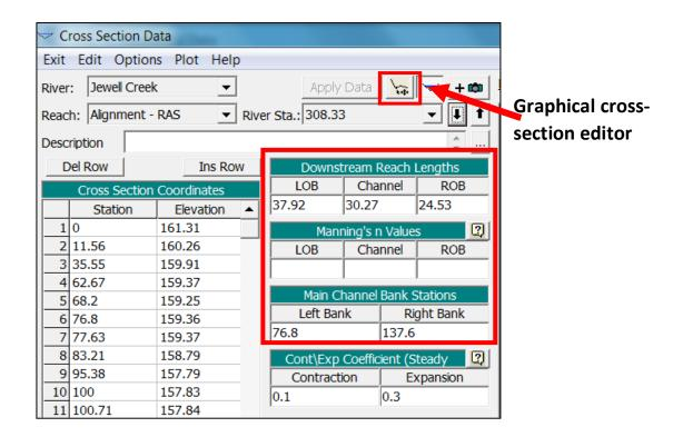
The locations where the reach length lines intersect the cross-sections is set to the bank station in RAS. Since generally we want the overbank flow reach length to be further out from the bank, these bank stations will need to be adjusted in RAS. It is most convenient to have Civil 3D compute all the flow reach lengths, and then in RAS move the bank stations, using the Graphical Cross-Section editor.
