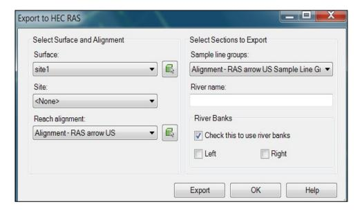
The geometry file created by CAD requires some manipulation before importing to RAS, in order for the stationing, bank sections and aesthetic flow direction arrow to all be correct. There's a spreadsheet macro – RASflipper - that takes a .geo file of RAS data exported from Civil 3D and flips it around so that it imports correctly into HEC RAS. It's available here:
