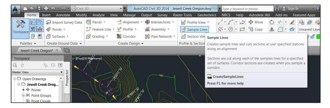
In the Create Sample Line Group window, name the sample line group and select the surface you want to sample from, if you have multiple surfaces. Uncheck the Sample box for a surface if you do not want to sample from that surface.
