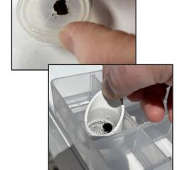
Another easy method is the bottle cap test. This is done similarly to the simple field method above. Placing a soil fragment or 'ped' in a water bottle cap full of water. After 30 seconds, swirl the water in the bottle cap for 5 seconds. If the soil stays intact, you have good aggregate stability, but if the soil breaks apart during agitation or within the first 30 seconds, you may have low stability.
