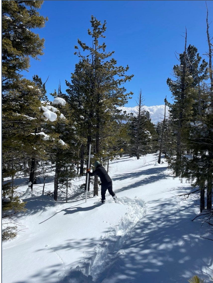
Janella Cruz, NRCS Resource Soil Scientist, measures a point along the Aztec #2 Manual Snow Course in the Canadian Basin near Cimarron on March 27 th , 2024. This site held 21 inches of Snow Depth and 3.1 inches of SWE on the survey date. This value represents 123% of the reference period normal SWE. NRCS Photo: Jaz Ammon.
