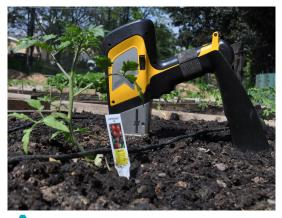
The portable X-Ray Fluorescence (pXRF) soil screening can determine the concentration of lead and other trace metals on-site; the spatial variability and presence of any "hot spots," and whether there is a need for consideration on a different use and/or management.
