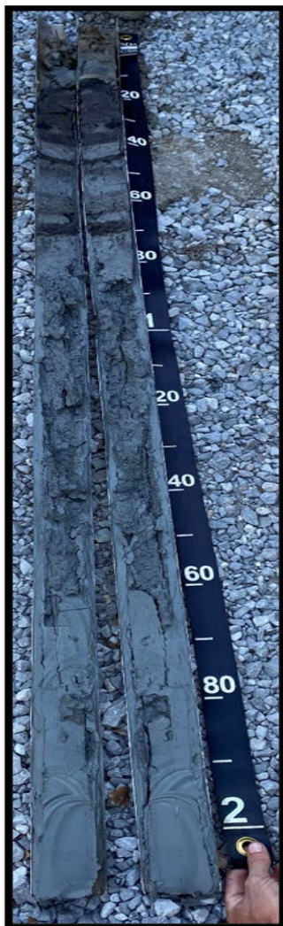
Figure 2.—Vibracore sample open and ready to be described.
