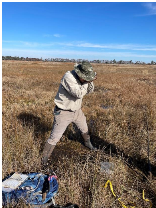
Image 1.—Braden Fleming listens for a reaction to 30% hydrogen peroxide to indicate the presence of reduced sulfides during a confirmation description.
