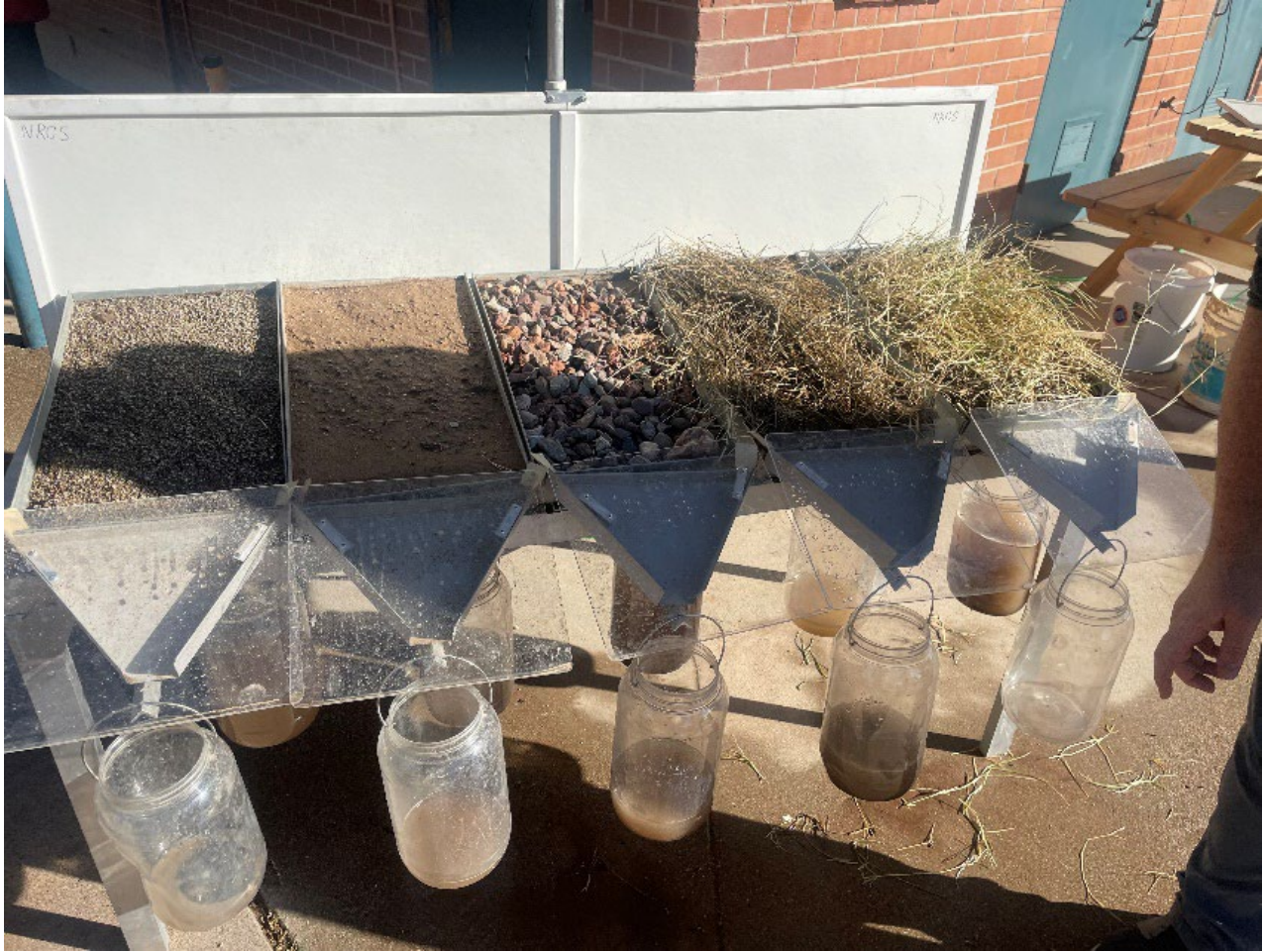
Figure 1.—Demonstration of different substrate cover types and how they impact soil runoff or erosion and water infiltration.
