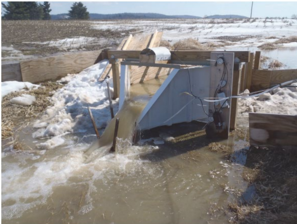
Monitoring station at the inlet of the water and sediment control basin (WAS1) during a December 2014 rain-on-snow event
