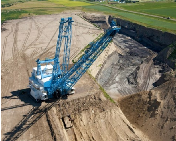
2023 — One of the draglines at the Coteau Freedom Mine near Beulah, ND. The bucket capacity is 124 cubic yards, which is enough space to park 3 Chevy Suburbans (photo courtesy of Basin Electric Power Cooperative).
