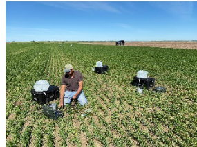
Ksat data collection with SATURO ® units at the No-till small grain-fallow field.
