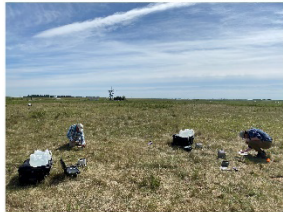
USDA staff conducting sorptivity tests and collecting Ksat data with SATURO ® units at the moderately grazed pasture.
