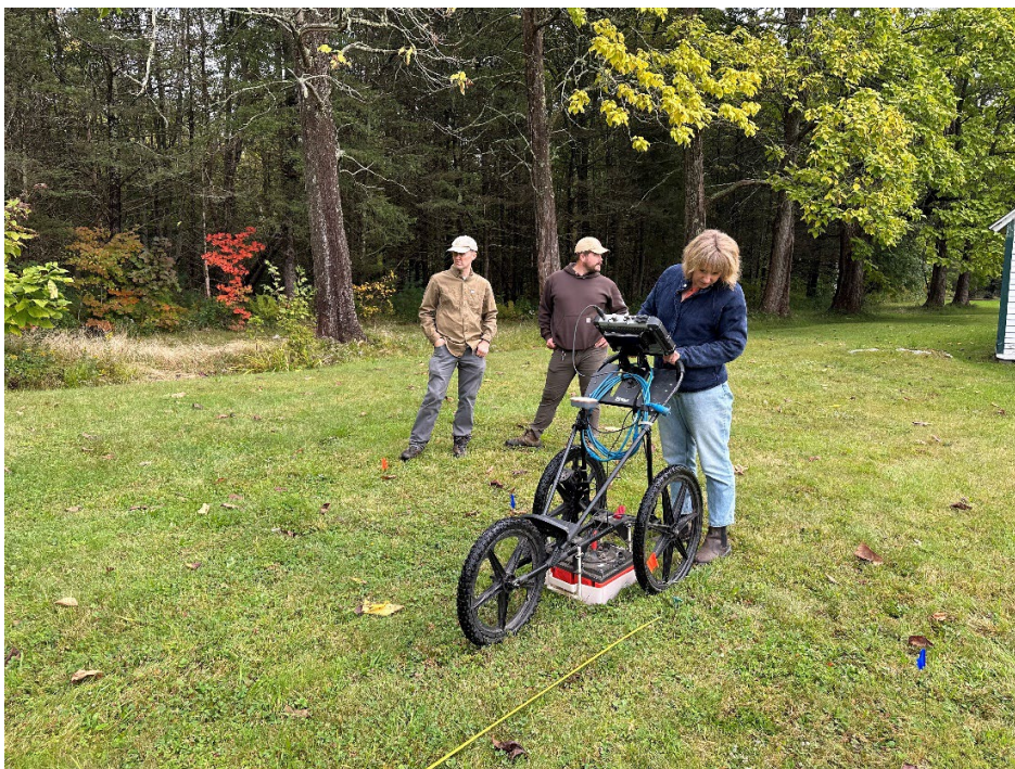
Figure 1.—NRCS staff conducting the GPR grid survey.
