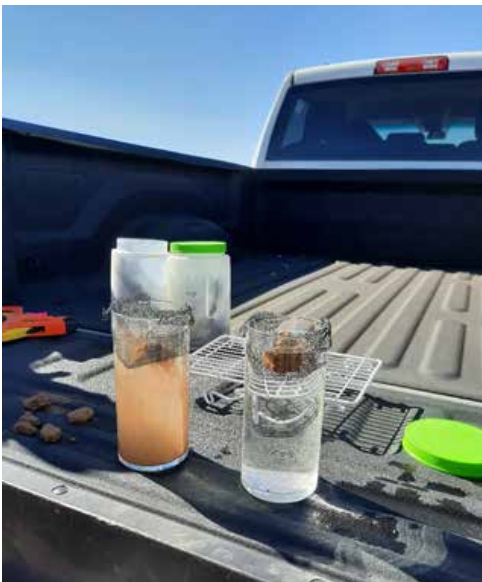
A slake Test as part of a Cropland In-Field Soil Health Assessment training near Fence Lake.
