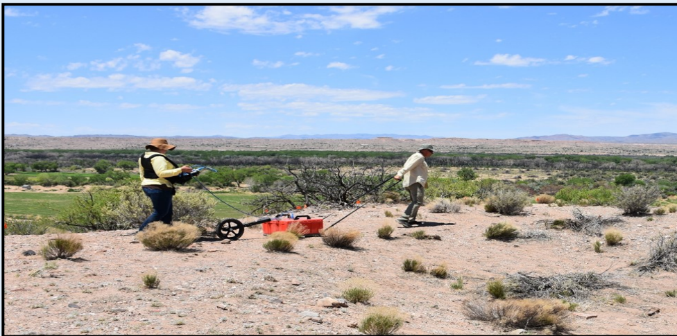
NRCS Archeologist and Soil Scientist –Geophysics conducting a Ground Penetrating Radar survey.
