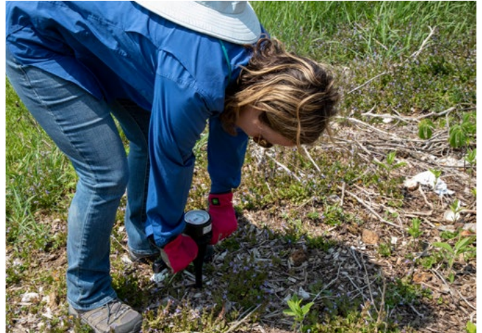
Hillary Olson, NRCS State Soil Health Specialist uses a penetrometer to test the extent and depth of subsurface compaction in Alisha Sedlmayr's garden.
