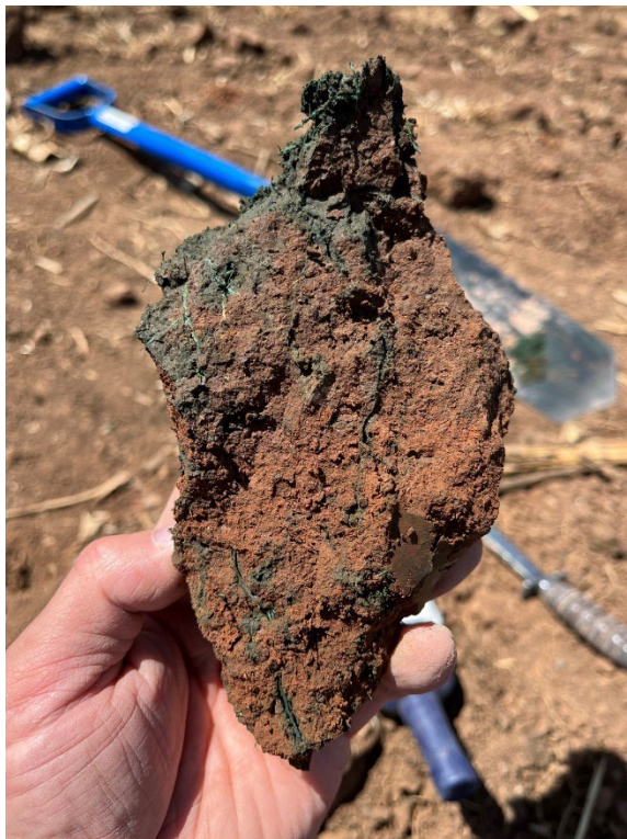
A close-up of a soil ped showing blue dye in the root channels.
