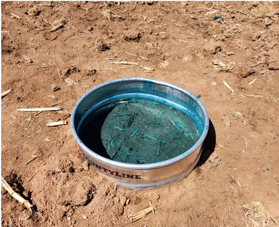
The infiltration study used a galvanized fire pit ring, blue food coloring, and 30 gallons of water to demonstrate water movement through the soil. The colored water was allowed to saturate the surface and soak into the ground for three days.
