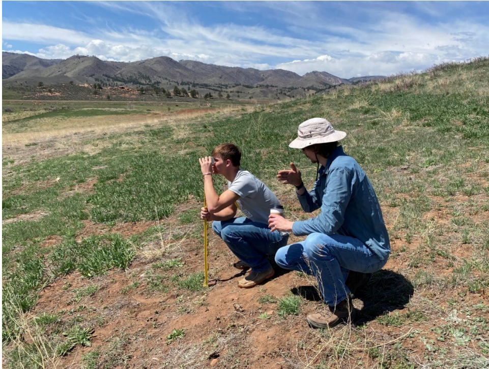
Matt Wellick, SPSP Soil Scientist, explains how to use a clinometer to an FFA contestant. Some students do not have prior experience measuring slope with a clinometer.
