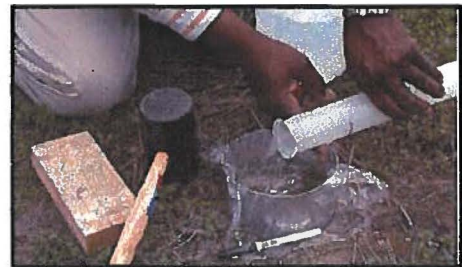
Figure 7: Preparing soil infiltration test
