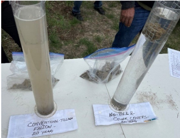
Figure 3. The slake test demonstration showed some of the differences between soils under conventional till (left) and no-till (right) (Photo by Scott River Watershed Council staff).
