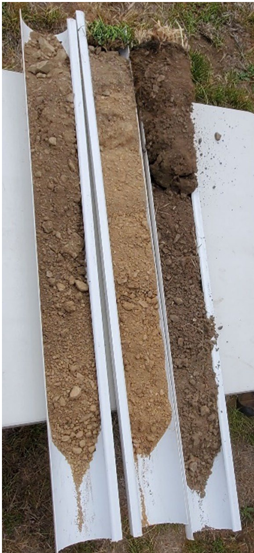
Figure 1. Soil cores of the Stoner soil series under different management scenarios (left to right: annually tilled grass hay; alfalfa hay; no-till pasture with biochar amendments).
