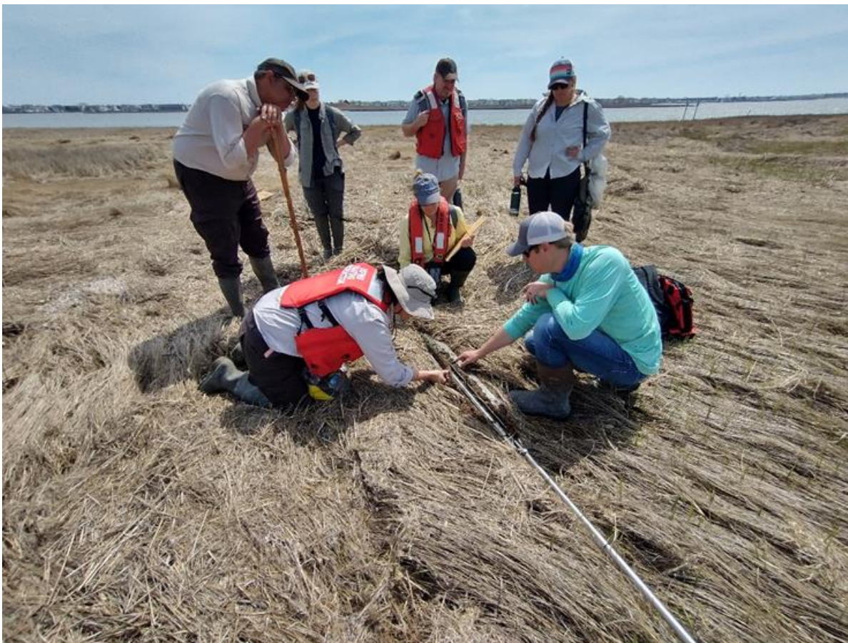
Figure 1. SSO Leader, David Steinmann (right), describes and explains the soil profile from a Macauley auger to the project team. The soil is a Pawcatuck series, a Terric Sulphemists. (Photo courtesy of Bill Shadel, The Nature Conservancy.)
