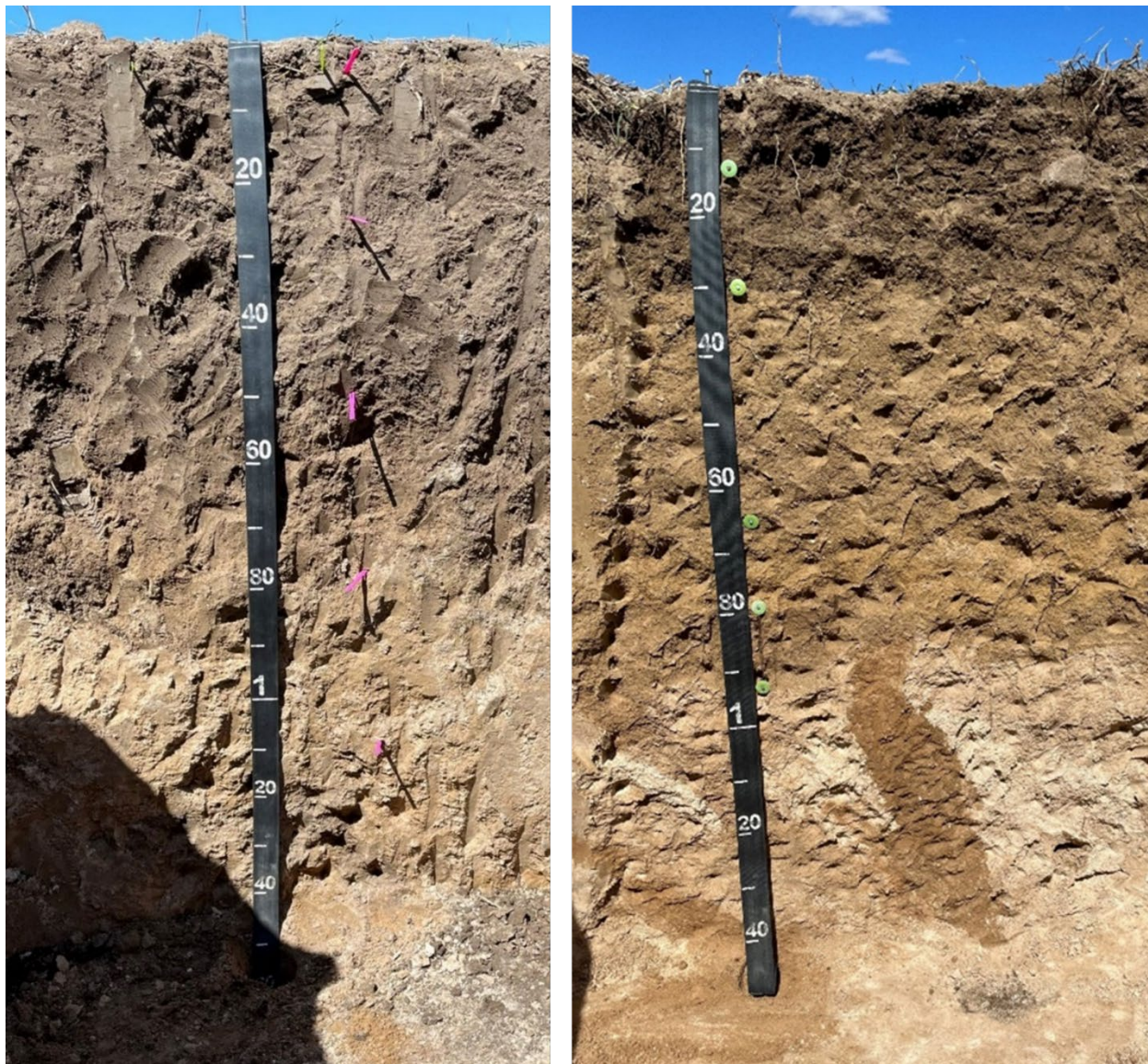
Figure 3. Soil profile of the soil characterization and agriculture soil pit, a fine-loamy, mixed, superactive, mesic Pachic Argiustolls (left). Soil profile of the homesite soil pit, a coarse-loamy, mixed, superactive, mesic Aridic Calcistolls; notice the large krotovina from 90 to 140 cm (right). (Photos by Andy Steinert).
