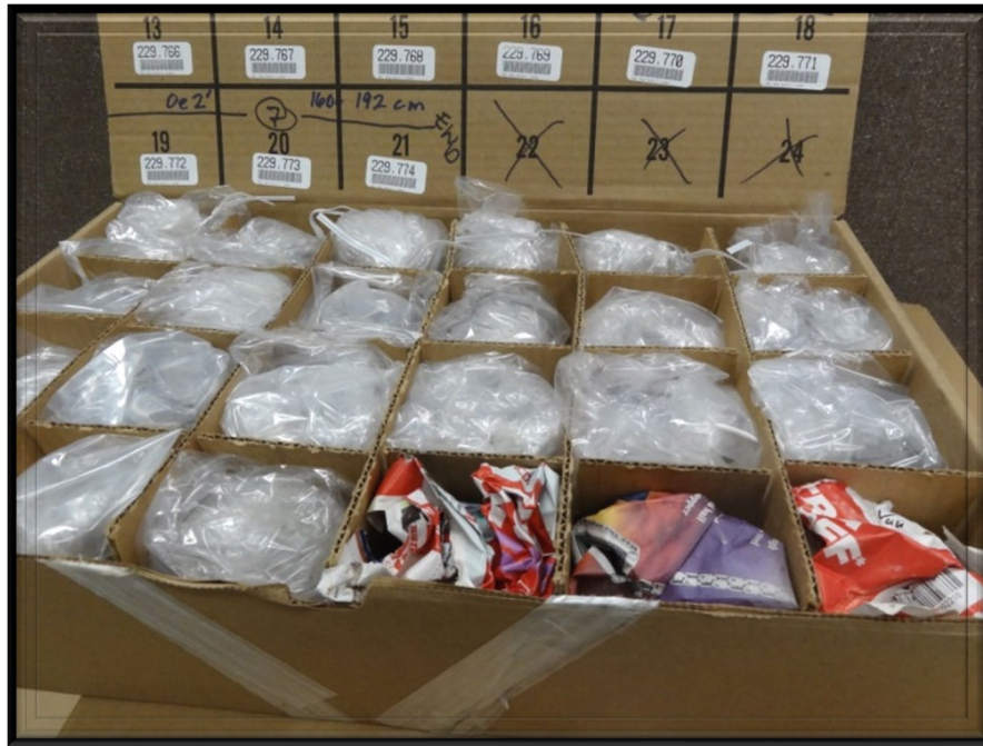
Figure 11.—A clod box in which the empty cells have been filled with packing material to increase stability. (Step 24)
