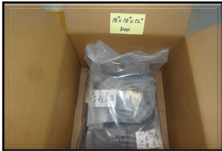
Figure 5.—A single secondary plastic bag in an 18" x 18" x 12" cardboard box furnished by the KSSL for bulk samples. (Step 12)
