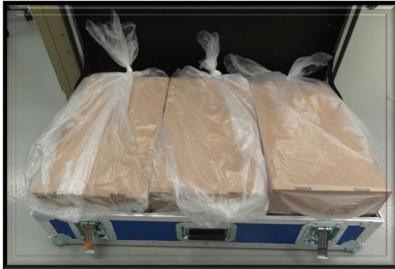
Figure 13.—Clod boxes in a clod trunk, which is furnished by the KSSL. (Step 27)
