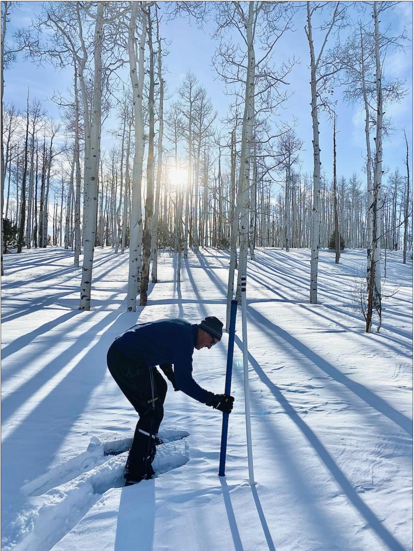
Doug Neff, Electronics Technician for the Utah Snow Survey, at the Fish Lake snow course obtaining manual readings of snow water equivalent (SWE) and snow depth for this year's April 1 report. Eight inches of SWE were measured at the site, which is not nearly the highest on record for April 1 st (22.4" were measured in 1984). It's fascinating how our snowpack is setting records in many places but isn't particularly noteworthy in other spots. This snow course has been continuously measured since 1931. Photo by Joel Burley.
