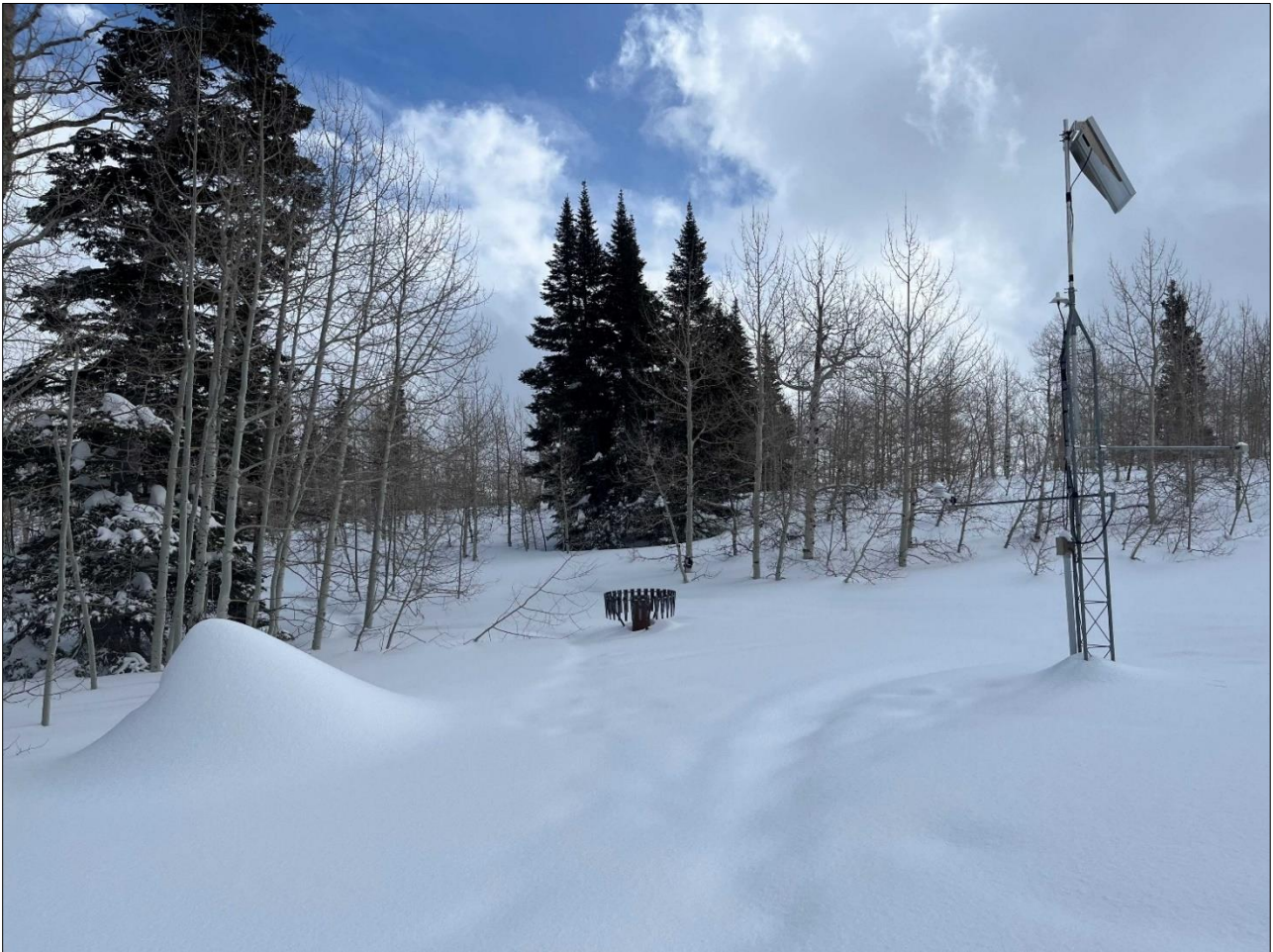
Timpanogos Divide SNOTEL site. The snow depth was 132" deep at the time this photo was taken, which almost reached the top of the precipitation can. The instrument shelter is the lump of snow on the left side of the image above. Shown below is Dave Eiriksson looking up from the instrument shelter after digging down to it to access the fluid manometer readings. A snow course preceded the existing SNOTEL site at this location and was measured from 1935 until the SNOTEL site was installed in 1978. This year's snowpack is the deepest ever recorded at this location on April 1, by a significant margin. Photos by Kent Sutcliffe.
