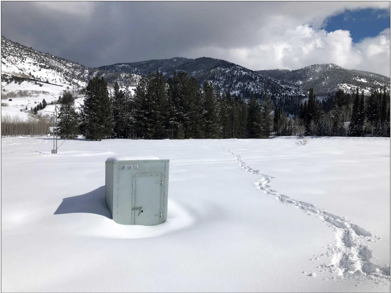
Tony Grove RS SNOTEL site, with the historic snow course in the distance. Data from this location date all the way back to 1924, making this the longest continuously measured snow measurement site in Utah. Manual readings of snow water equivalent (SWE) and snow depth were compared with automated values from the SNOTEL site for this year's April 1 report. Nineteen inches of SWE were measured at the site's snow course this year, which is the 4 th highest on record, surpassed only by 1936, 2011, and 1952. Photo by Jordan Clayton.
