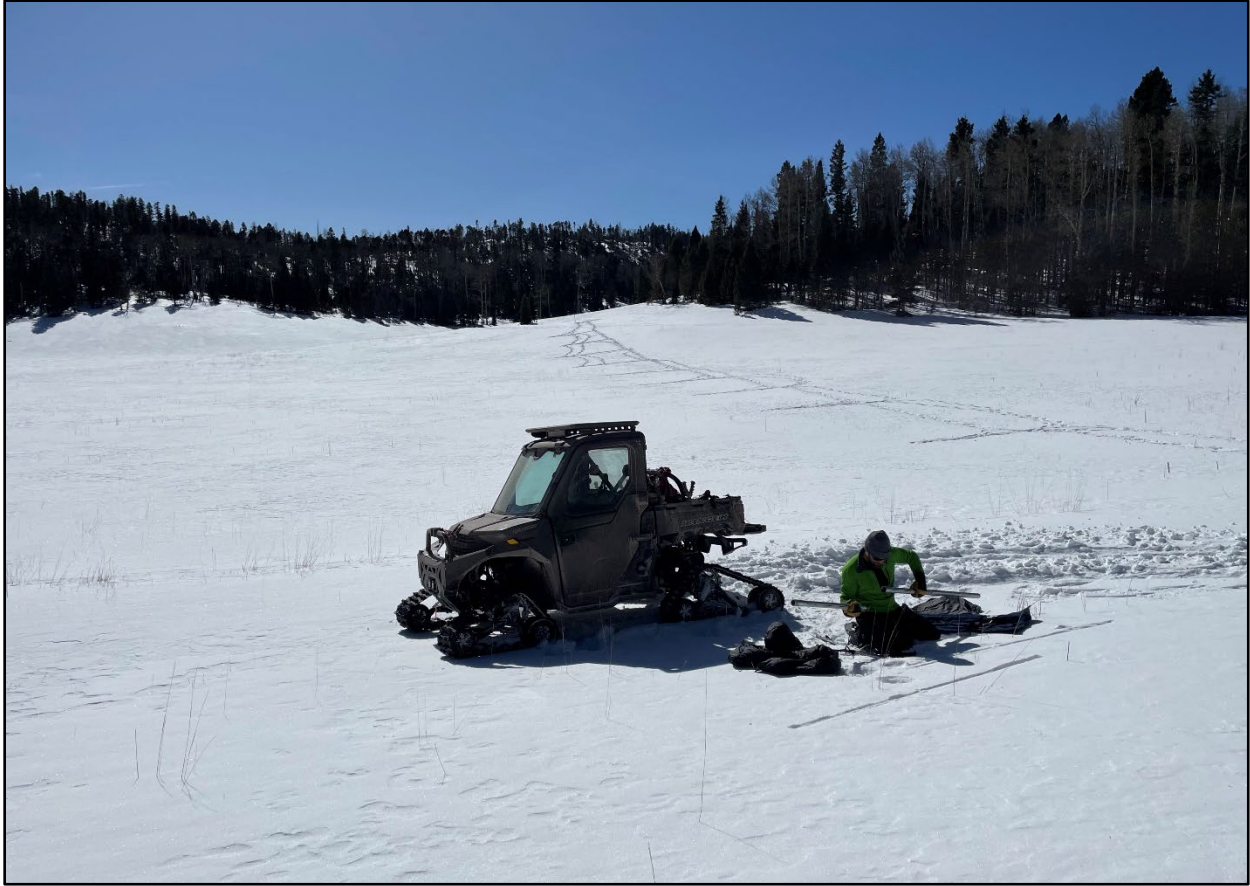
Logan Peterson, NRCS Soil Scientist, assembles a snow sampling kit at the Hematite Park manual snow course in the Canadian Basin on March 28 th , 2023. SWE at this site measured 153% of the reference period normal for the April 1 survey cycle. NRCS Photo: Jaz Ammon
