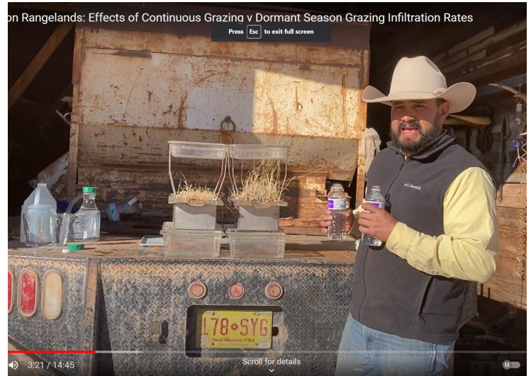
NRCS State Rangeland Management Specialist demonstrates the Effects of Rainfall on a healthy vs. unhealthy land using Rainfall simulator in a YouTube video (Winter 2022).
