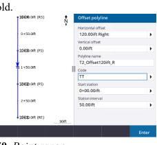
Layout the offset terrace alignment using a keyed in polyline.
