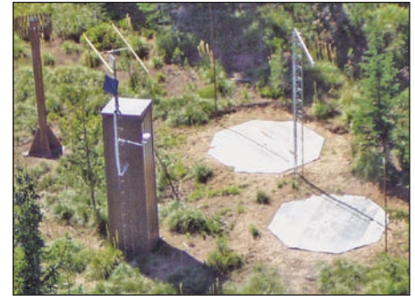
Crater Meadows SNOTEL site, Idaho. Hypalon snow pillows (white circles about 3 m in diameter) measure snow water equivalent and are the primary basis for most Western US water supply forecasts. Precipitation gauge is in upper left. Other instruments are mounted on the tower between the two snow pillows. All SNOTEL sites are solar powered.
